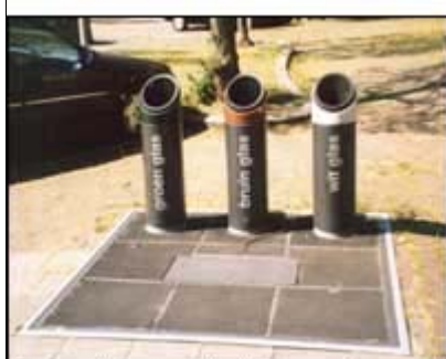
Underground glass recycling container (Dordrecht)
